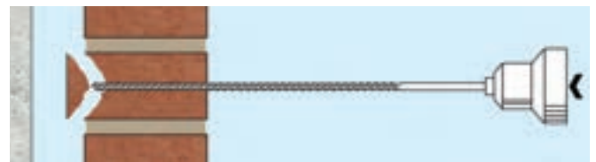
A. Do NOT use SDS type drill to drill the pilot hole
