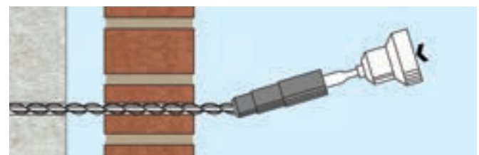
C. Do NOT drive tie in at an angle
